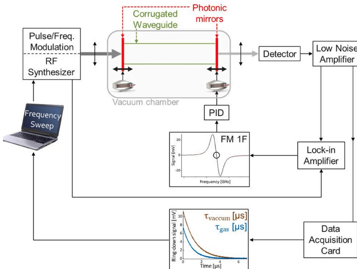
**Fig. 1.** THz cavity ring-down spectrometer. The emission of a microwave synthesiser and amplified multiplier chain is injected into the cavity. The ring-down signal is amplified by 60 dB with a bandwidth of 200 MHz. The DAQ samples and provides a real time average used to determine the ring-down time. The cavity length is locked to the emission frequency using piezo-electric actuators and a PID control loop.
