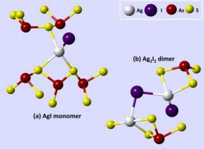
**Fig. 12.** Schematic representation of isolated AgY monomers or dimers in a disordered silver halide thioarsenate glass network in the critical percolation region based on initial RMC configuration of a  $(AgI)_{0.2}(As_2S_3)_{0.8}$  glass.
