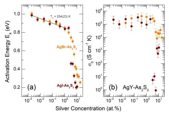
**Fig. 6.** (a) Conductivity activation energy  $E_a$  and (b) conductivity pre-exponential factor  $\sigma_0$  of ( $\bullet$ , orange) AgBr-As<sub>2</sub>S<sub>3</sub> and ( $\bullet$ , brown) AgI-As<sub>2</sub>S<sub>3</sub> glasses. The solid line represents a least-square fit of the  $E_a$  experimental data points in the critical percolation domain to Eq. (4).
