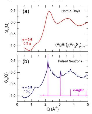
**Fig. 1.** A low-Q part of (a) the x-ray  $S_X(Q)$  and (b) neutron  $S_N(Q)$  structure factors for AgBr-rich thioarsenate glasses. A small y=0.6 glass sample (0.3 g) was used for high-energy x-ray diffraction experiments. A much larger y=0.5 sample (10 g) was measured using pulsed neutrons. Characteristic Bragg peaks of cubic AgBr, space group  $Fm\overline{3}m$  [23] are also shown.
