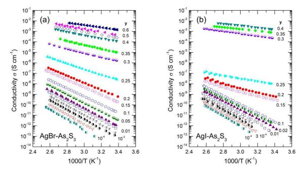
**Fig. 4.** Temperature dependences of the total electrical conductivity  $\sigma$  for the (a)  $(AgBr)_y(As_2S_3)_{1-y}$  and (b)  $(AgI)_y(As_2S_3)_{1-y}$  glass systems. The numbers for selected glasses indicate the AgY molar fraction y.
