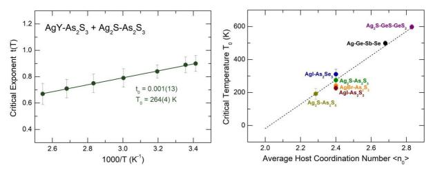
**Fig. 7.** Average values of the critical exponent t(T) calculated for AgY- and Ag<sub>2</sub>S-As<sub>2</sub>S<sub>3</sub> glasses at  $x \le 2$  at.% Ag and plotted as a function of reciprocal temperature. The derived  $t_0$  and  $T_0$  parameters are also shown.
