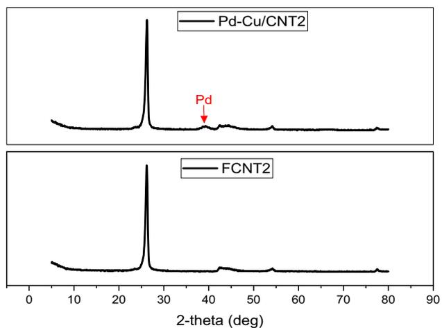
Figure 4: XRD patterns of FCNT2 and 4Pd-1Cu/FCNT2.
