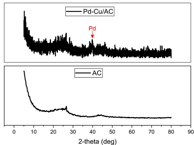
Figure 5: XRD patterns of AC and 4Pd-1Cu/AC.
