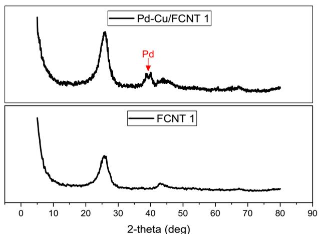
Figure 3: XRD patterns of FCNT1 and 4Pd-1Cu/FCNT1.
