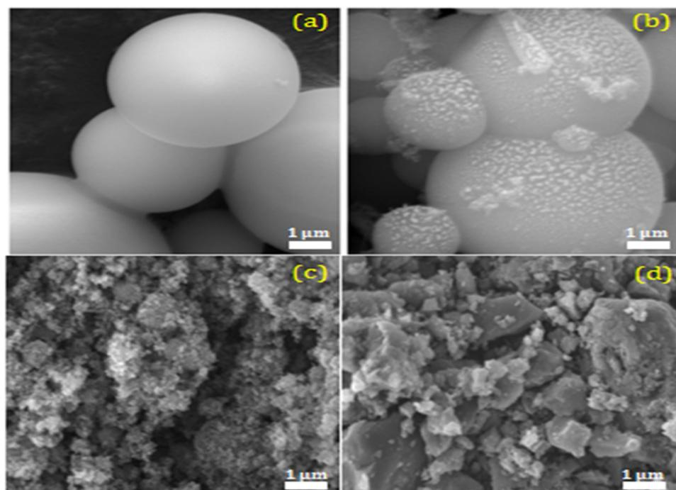
Figure 9: SEM images: (a) SBA-15, (b) 1Pd-1Cu/SBA-15, (c) TiO<sub>2</sub>, and (d) AC.
