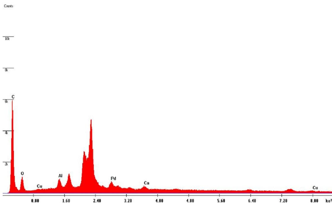
Figure 12: EDX pattern of 4Pd–1Cu/TiO<sub>2</sub>.
