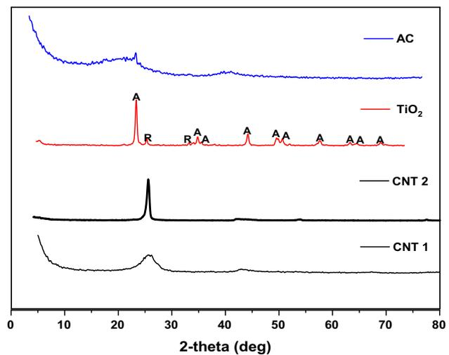
Figure 1: XRD patterns of CNT2, TiO<sub>2</sub>, CNT1, and AC.
