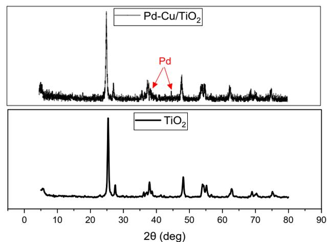
Figure 6: XRD patterns of  $\text{TiO}_2$  and 4Pd-1Cu/ $\text{TiO}_2$ .
