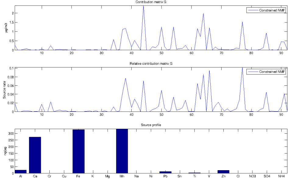
Figure 6: Ferromanganese plant source.
