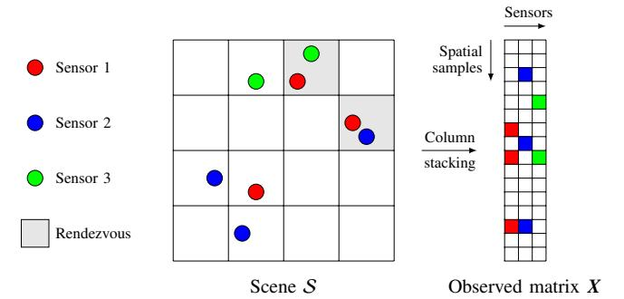
Fig. 1. From a scene  $\mathcal{S}$  (with  $n = 16$  spatial samples,  $m + 1 = 3$  sensors and 2 rendezvous) to the data matrix  $X$  (white pixels mean no observed value).
