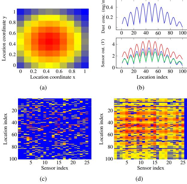
Fig. 2. (a) The  $10 \times 10$  simulated scene  $\mathcal{S}$  (pollution field); (b) (top) the vectorized scene  $\mathbf{y}$ , (bottom) three vectorized sensor readings of  $\mathbf{y}$ ; (c-d): simulated dataset with 25 mobile sensor and 4 reference measurements (in the last column of  $\mathbf{X}$ ) with (c)  $\rho_{MV} = 0.8$  and  $\rho_{RV} = 0.9$ ; (d)  $\rho_{MV} = 0.1$  and  $\rho_{RV} = 0.1$ .
