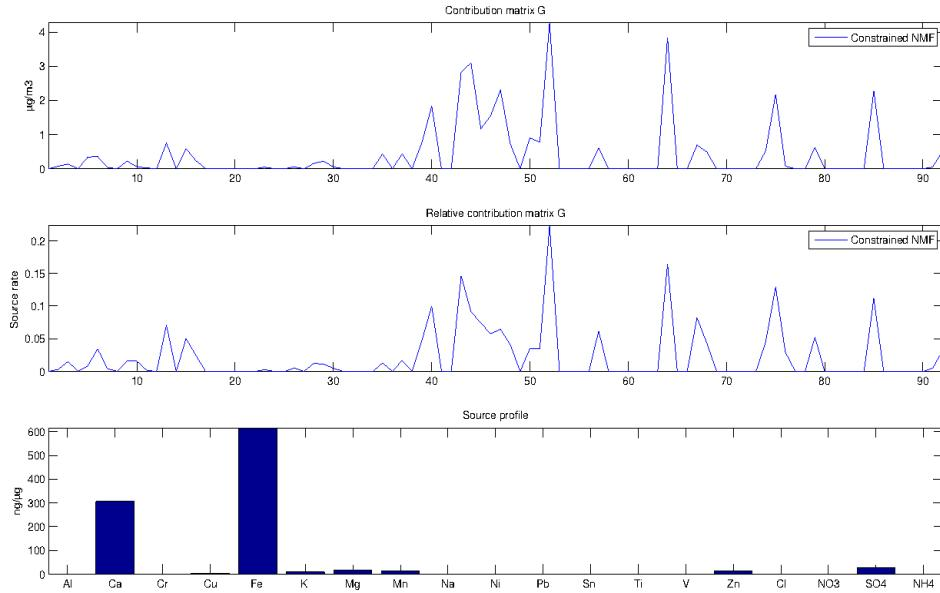
Figure 2: Blast furnaces source.
