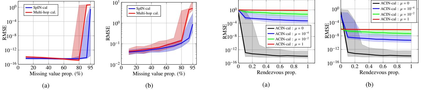
Fig. 7. Comparison of SpIN-cal with multi-hop calibration [16] with respect to the proportion of missing values in (a) noiseless and (b) noisy scenarios.
