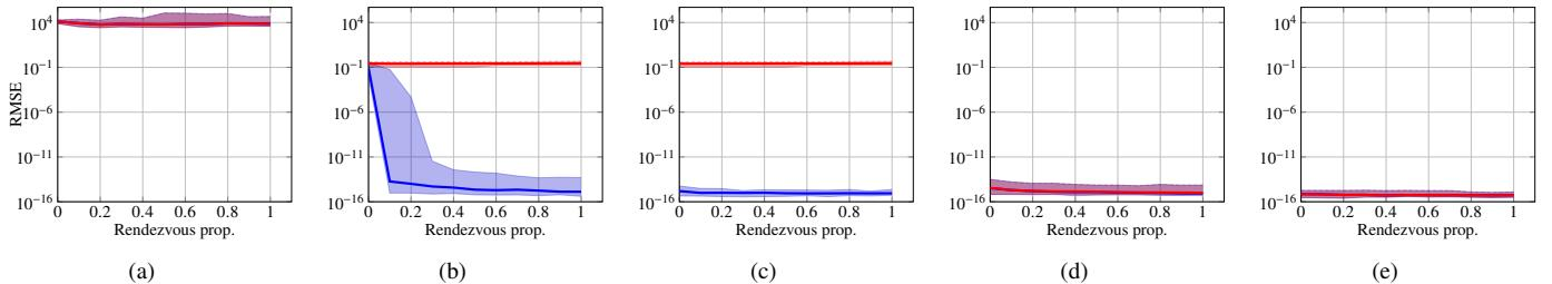
Fig. 9. Evolution of the  $\text{RMSE}_1$  (in blue) and  $\text{RMSE}_2$  (in red) with respect to the rendezvous proportion: (a) Natural approach; (b) IN-cal; (c) ACIN-cal; (d) SpIN-cal; (e) SpAIN-cal.
