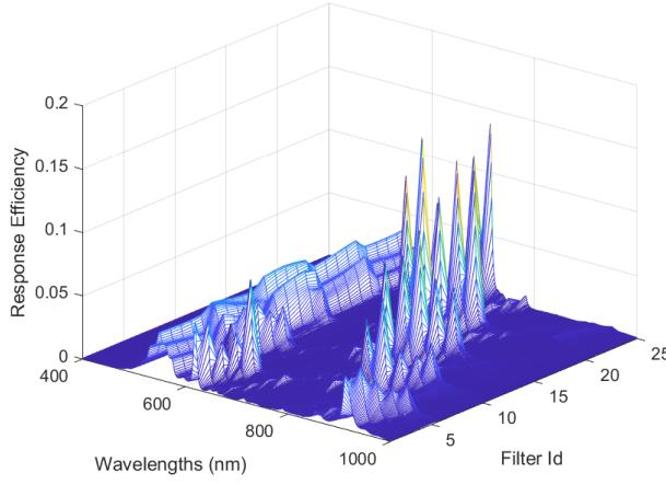
**Fig. 1.** Spectral response of the 25 spectral filters of the  $5 \times 5$  mosaic Photon Focus SSI camera in the 400–1000 nm range.
