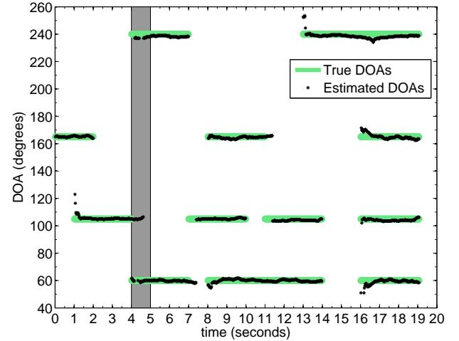
Fig. 8. Estimation of DOA of four intermittent speakers at  $60^\circ$ ,  $105^\circ$ ,  $165^\circ$ , and  $240^\circ$  in a simulated reverberant environment with 20 dB SNR and a one-second block size. The gray-shaded area denotes an example “transition period”.
